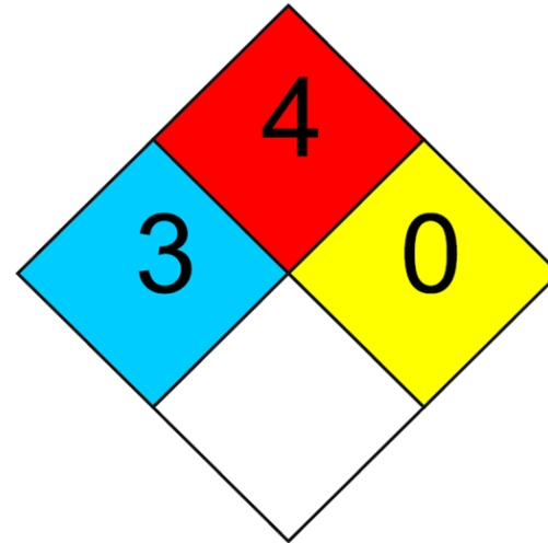
MAY BE FATAL IF INHALED. MAY CAUSE TARGET ORGAN DAMAGE, BASED ON ANIMAL DATA. FLAMMABLE GAS. MAY CAUSE FLASH FIRE.
