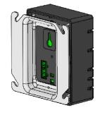
digital, Modbus signal. A unique address created for each of the gas detectors by using an 8 bit DIP switch on the MRS-485 adaptor. The MRS-485 adapters are wired in series, sometimes called a daisy-chain, using shielded 3-conductor wire with one twisted pair providing a pair for signal (A & B), common (COM) and shield ground (SHD) connections.
