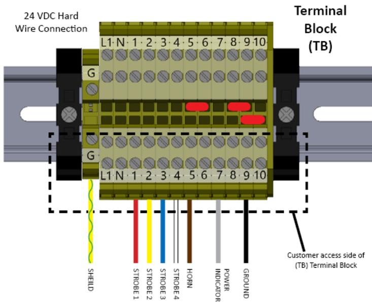
Figure 3-2 – Terminal Block connections
