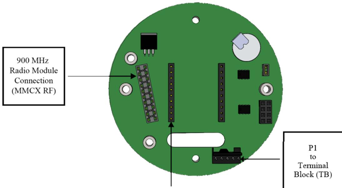
Figure 4-12 – Display/Radio Board (83-8008-0000-00)
