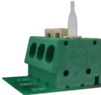
3. Insert the bare wire into the respective wire cavity of the connector. Refer Table 3-2.
