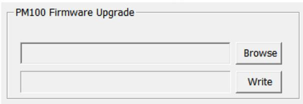
The Bump-Calibration Station can be used to upgrade the PM100 firmware. The Bump-Calibration Station can keep a copy of the PM100 firmware saved on its USB Disk. If there is a new firmware version, the file can be found at <https://macurco.com/downloads/>.
