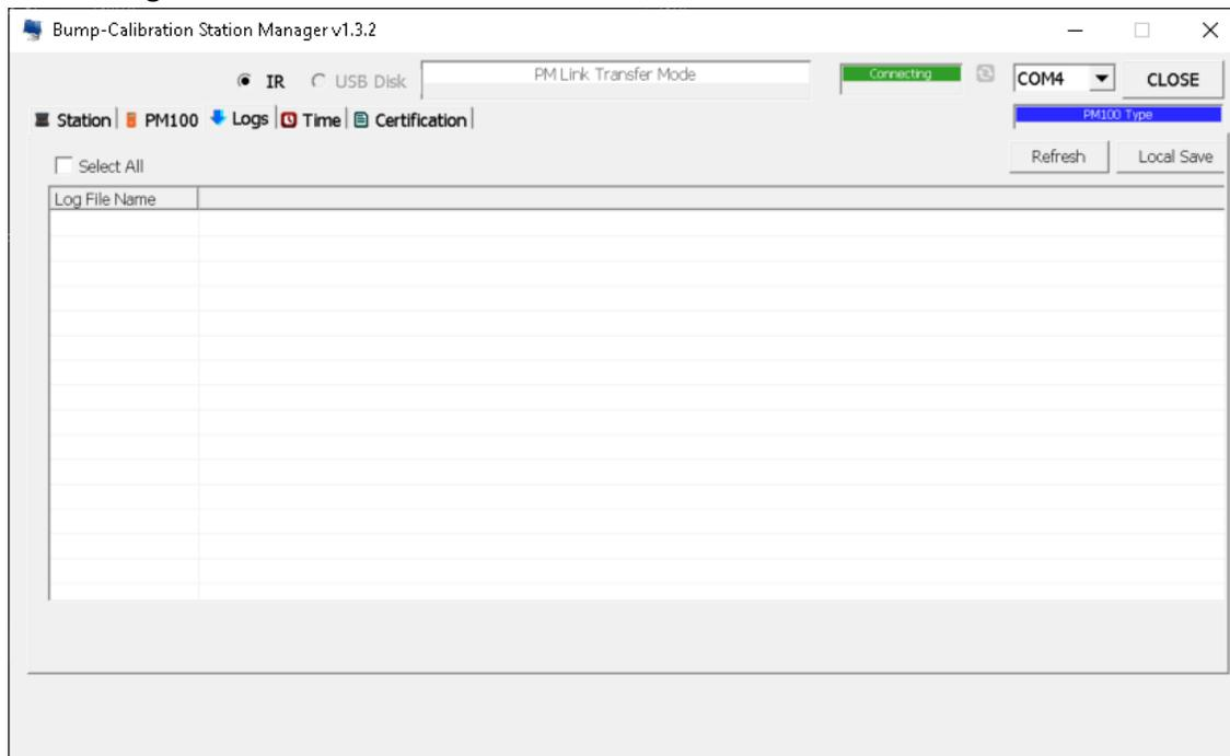
Logs are stored on the USB Disk and can be viewed on a computer using the Bump-Calibration Station Manager software. The log files will be formatted as .csv files (comma separated values) for easy viewing and manipulation with spreadsheet software. A log file will be created for each PM100 monitor used in the Bump-Calibration Station. A single log file will be created for the Bump-Calibration Station.
