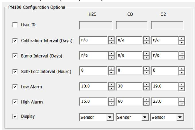
Each of the following configuration options can be enabled/disabled using the checkbox on the left side.
