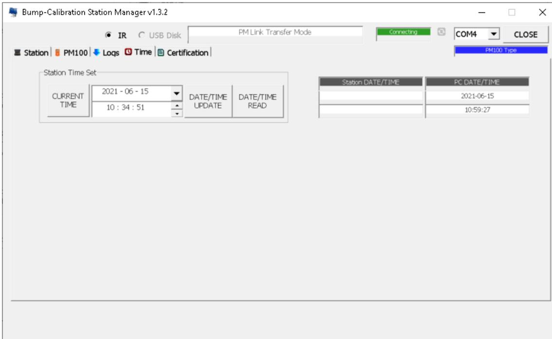
The Bump-Calibration Station adds time data to all its logs. If the Bump-Calibration Station time is incorrect, it can easily be updated to the correct time using the Bump-Calibration Station Manager software. The time can only be set when connected using the PM Link.
