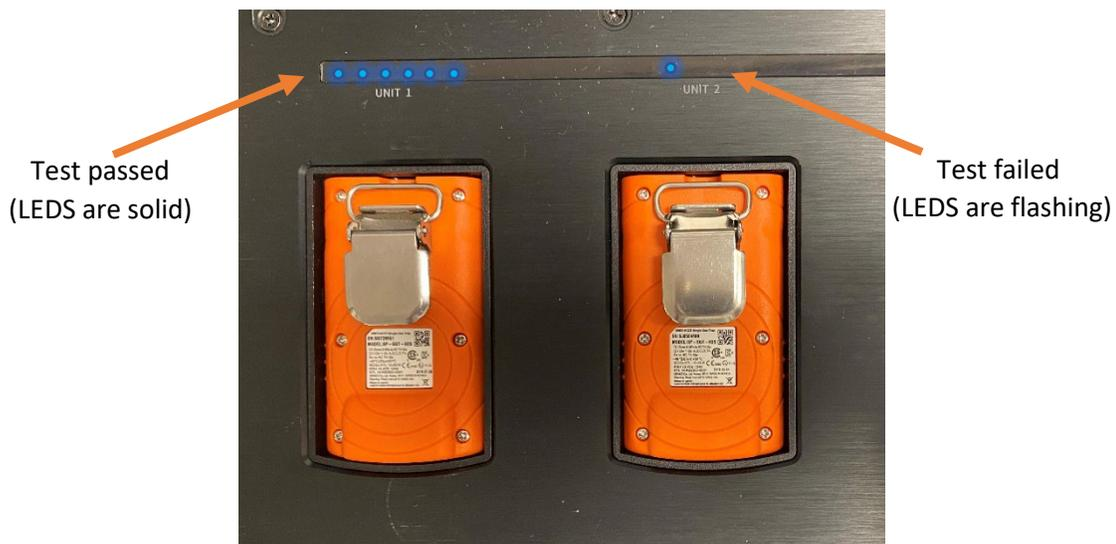
Figure 4–1 LED pattern indicates test pass or fail
