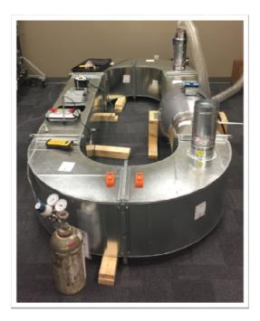
A Macurco Trac-XP Model TXP-T40 was calibrated and used as a control in the carbon monoxide air duct tunnel.
