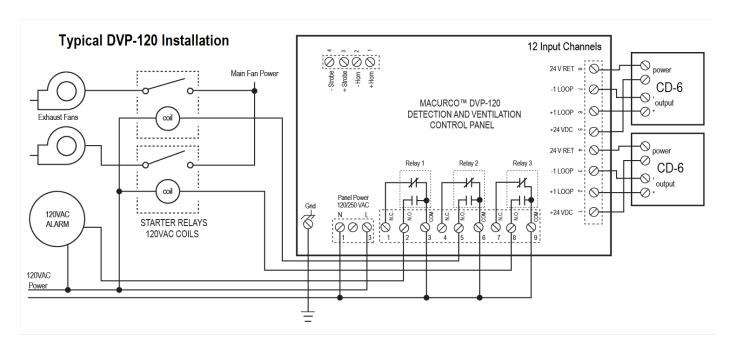
Figure 3-6 6-Series DVP-120 Control Panel
