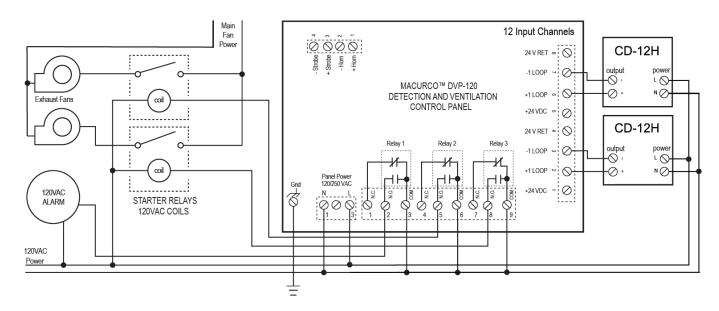
Figure 3-13 12-Series DVP-120 Control Panel
