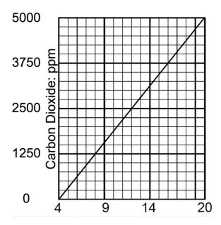
Figure 3-1 6-Series 4-20 mA Output diagram
