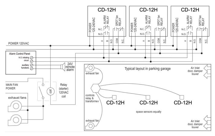
Figure 3-12 12 Series Alarm Control Panel diagram
