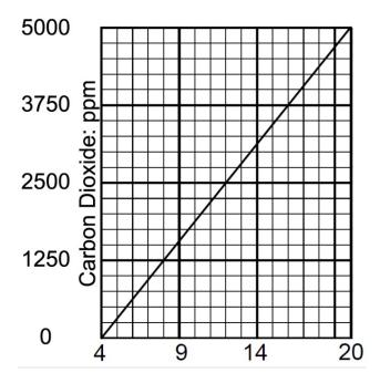
Figure 3-9 12-Series 4-20 mA Output diagram
