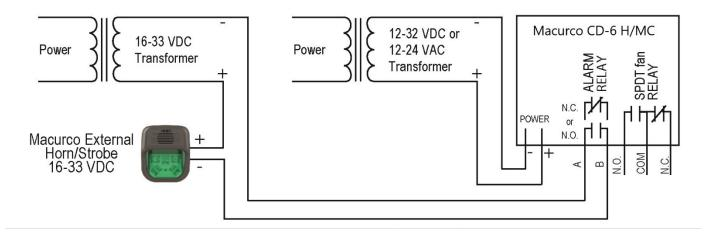
Figure 3-8 6-Series Horn & Strobe Combo Wiring
