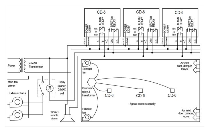
Figure 3-4 6-Series Multiple Device diagram
