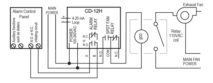
Figure 3-11 12-Series Alarm Control Panel
