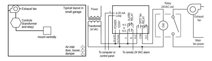
Figure 3-3 6-Series typical installation diagram
