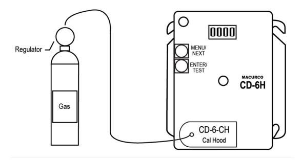
Figure 7-1 Calibration Connection
