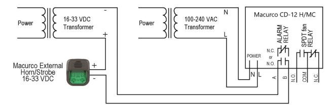
Figure 3-15 12-Series Horn & Strobe Combo Wiring
