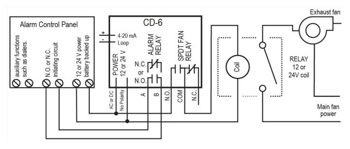
Figure 3-5 6-Series Alarm Control Panel diagram
