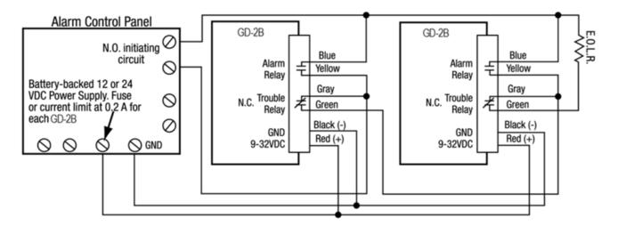
Figure 2 – Single Unit Wiring
