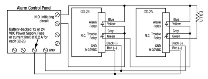
Figure 1 – Multiple Unit Wiring
